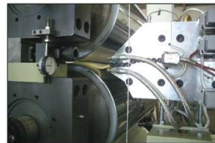
滾輪間隙採三角墊塊調整間隙。 Gap adjust between roller adopts triangular pad.
